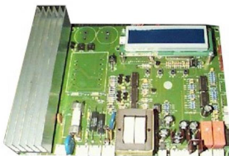
Combined digital control and alarm board
